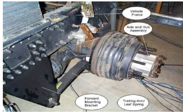
Fig. 2.4 VOAS-2 Suspension on test vehicle.
